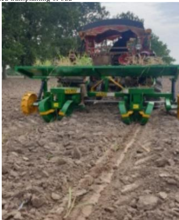
Fig. 2: The implement in the figure is the rear view of mechanical transplanter that maintain constant row to row distance in the field and plant sugarcane seedlings 3 inches deep in the soil.
