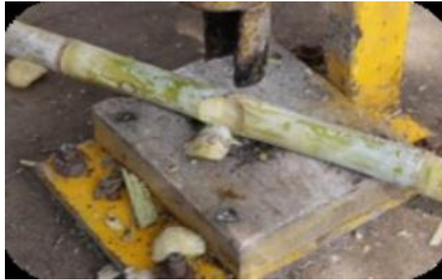
Fig. 3: Mechanical bud chip cutter having sharp U shape blade that cuts the bud with small chip from the sugarcane in the proper and simple manner, which allows individuals to use easily.
