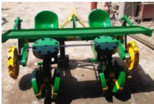
Fig. 1: Local modified, designed and manufactured sugarcane transplanter. The implement in the figure is the front view of mechanical transplanter that supports bud chip sugarcane planting technology.
